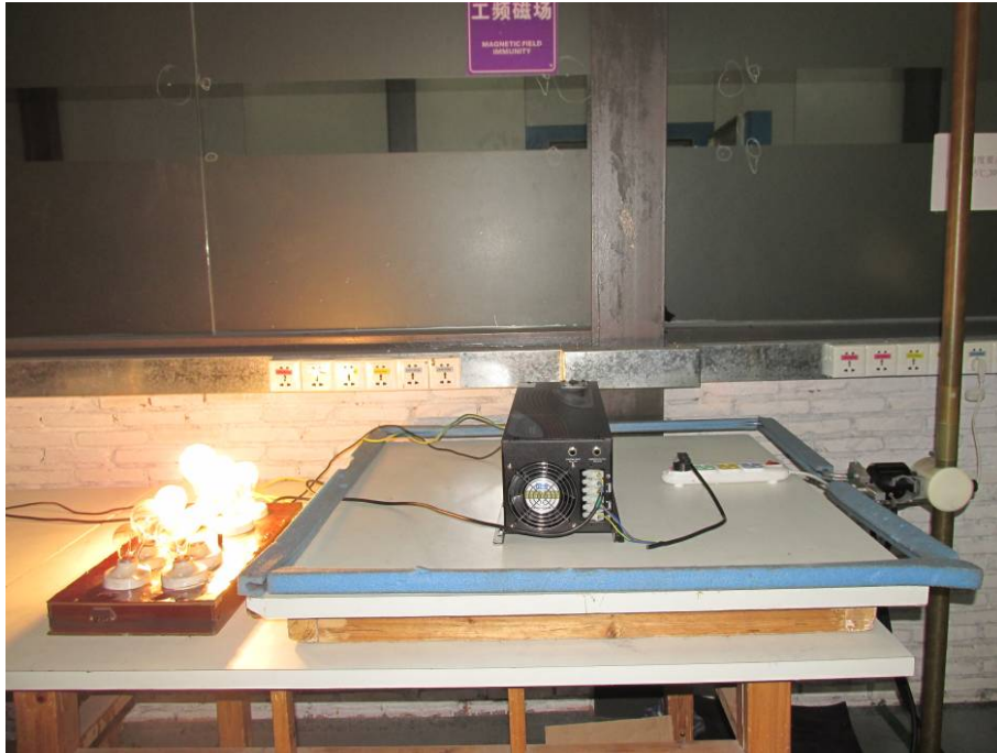
16.9. Photo of Magnetic Field Immunity Test
